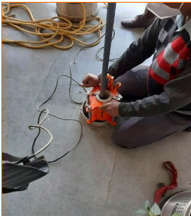
Scanning of Mine winder rope in progress at IMFA, Ltd, Jajpur, Odisha, with all safety precautions As a part of Non-destructive study – Visual inspection in progress to observe any defect(s) on surface of steel wire rope at Dewas, M.P.
