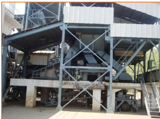
Figure : Pilot scale crushers for crushing the ROM coal to a suitable top size
