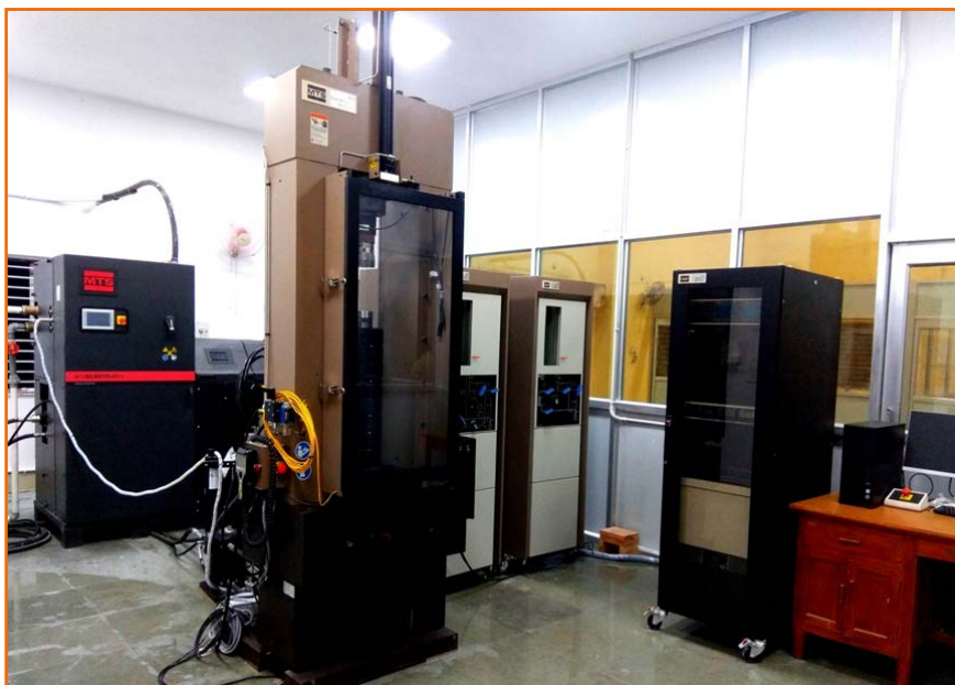
Figure 2: MTS 815 Rock Testing System (Load frame height is 2337 mm)
