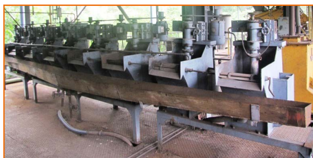
Figure : 400 kg/hr pilot scale flotation plant
