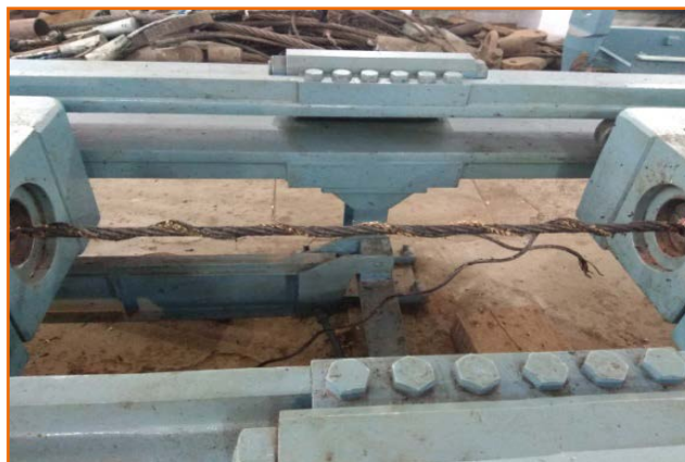
Laboratory Test of Wire Rope at 500t Horizontal Tensile Testing Machine
