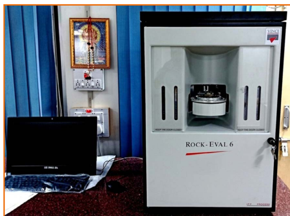
Figure 7: Rock-Eval 6 device installed at the CSIR-CIMFR Dhanbad
